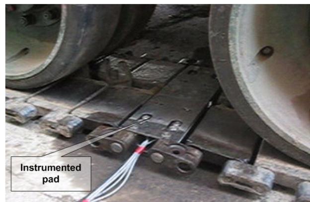
Figure 7 View of the instrumented pad inserted into the vehicle track
