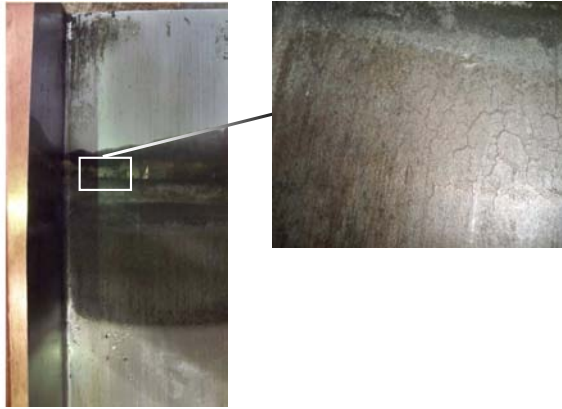
Figure 2. Inner mould surface with closed view of the meniscus region with cracks
