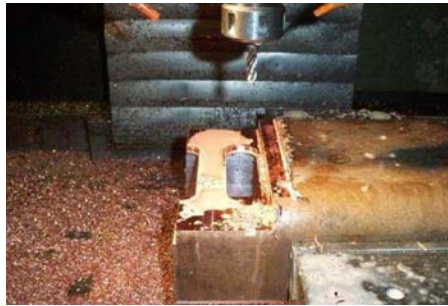
Figure 3. Manufacturing operation to obtain the tensile-test specimens.
