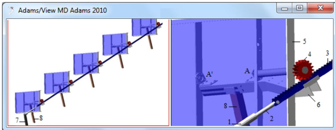
Fig. 1: The tracking mechanism for the PV string (ADAMS).
