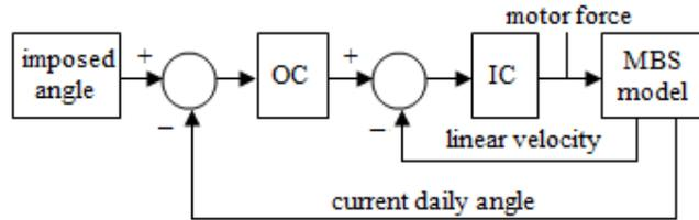
Fig. 2: The cascade control system.
