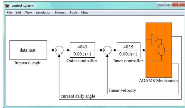
Fig. 3: The block diagram of the control system (MATLAB).
