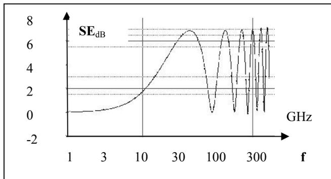
Figure 5: The material attenuation in the frequency range of 1GHz - 500GHz
