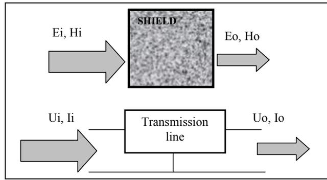
**Figure 1:** Lossless Transmission line model showing material properties
