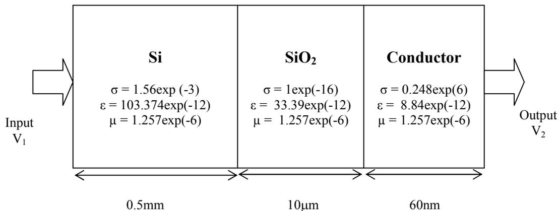
**Figure 3:** About the composite material construction
