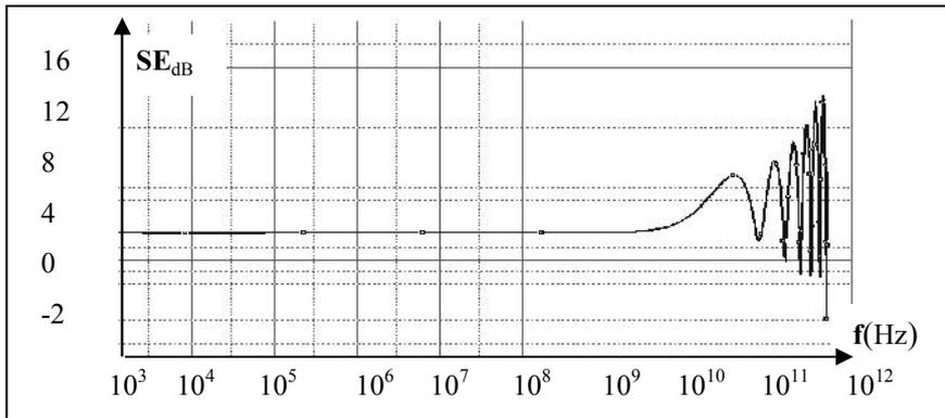
Figure 7: Simulation results taking into account a conductive layer of 60 $\mu$ m
