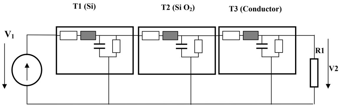
Figure 4: Layered composite material transmission line model
