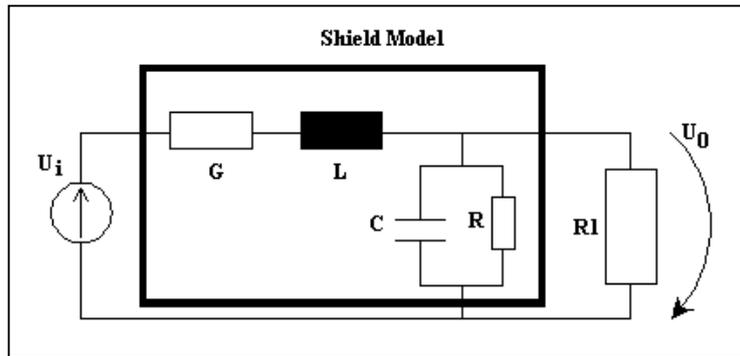
**Figure 2:** SPICE Model using the transmission line model for the studied material
