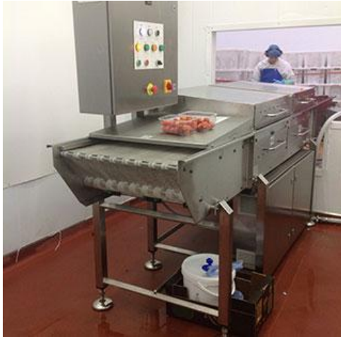
Figure 7: Decontamination tunnel produced by UV TECHNOLOGY LIMITED [11]
