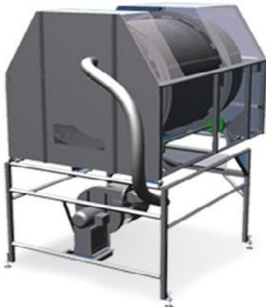
Figure 8: The UV-C Trumbling Drum decontamination equipment produced by REYCO SYSTEMS [12]
