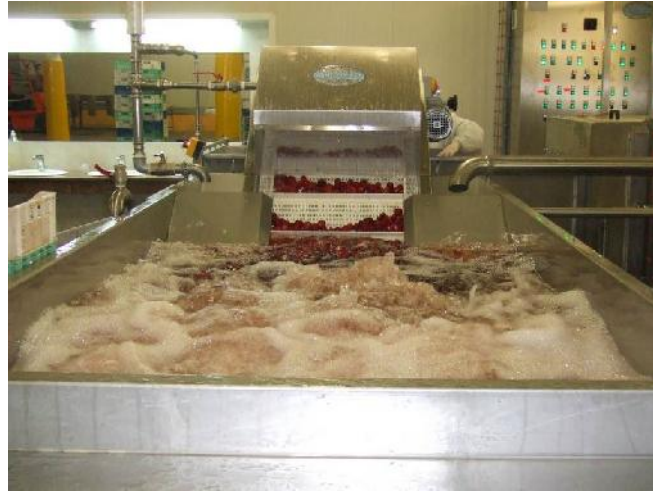
Figure 1: Washing tank with elevator manufactured by CESARE TAVALAZZI, Italy [3]
