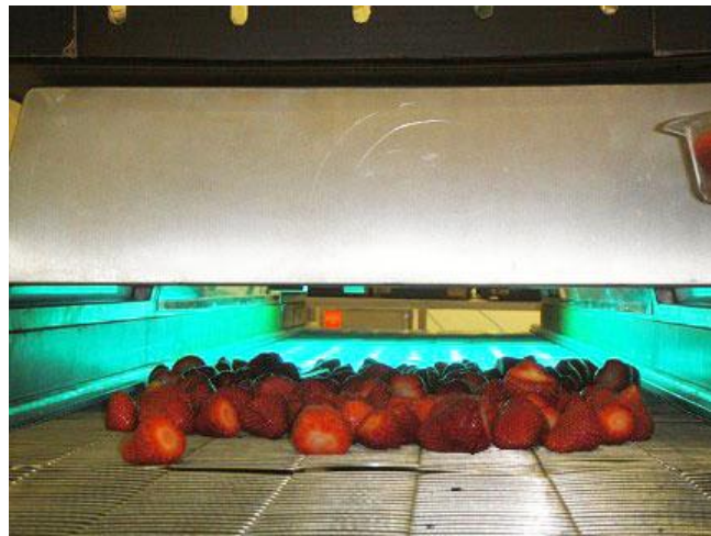
Figure 7: Decontamination tunnel produced by UV TECHNOLOGY LIMITED [11]
