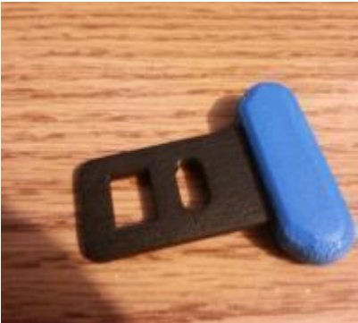
Figure 3: Tongue produced using a 3D printer
