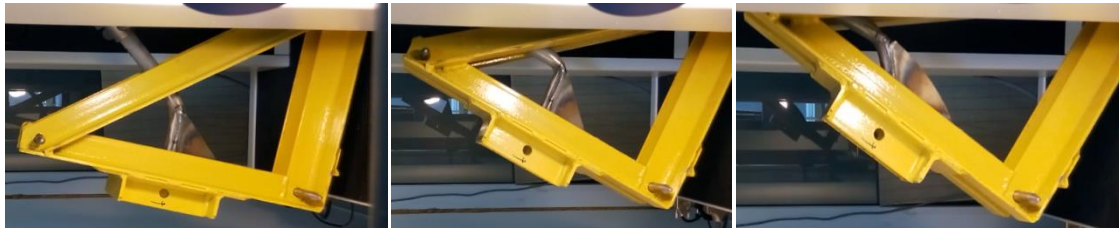
Figure 9: Joint gusset sample tensile testing
