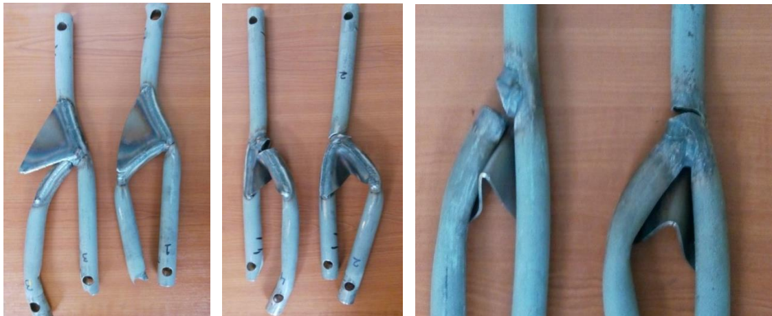
Figure 11: Tensile and compression subjected joint gusset samples
