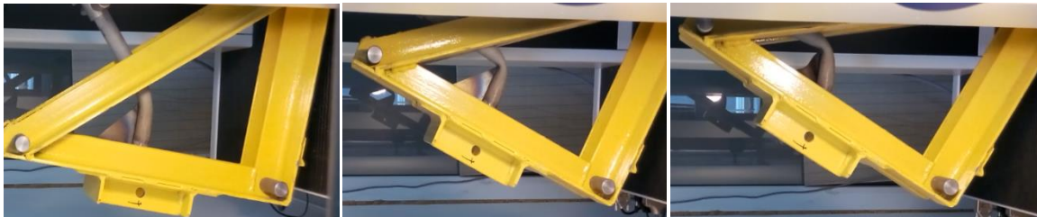
Figure 10: Joint gusset sample compression testing
