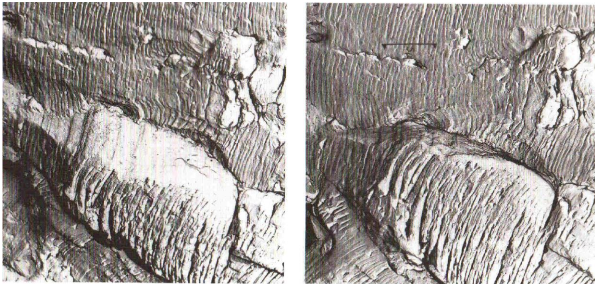
Figure 1a: A fatigue crack surface in Al-alloy
