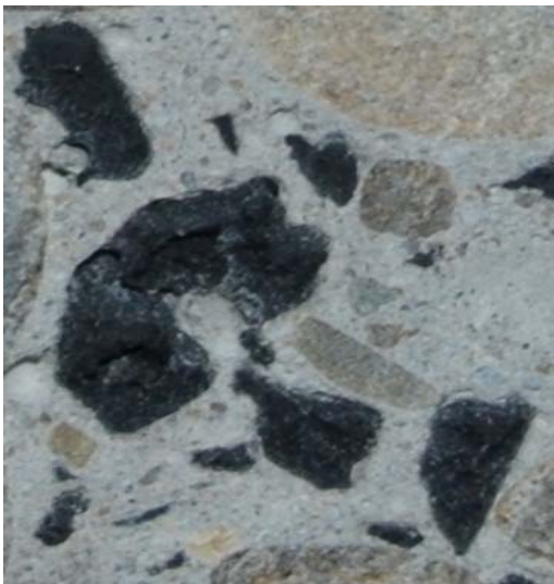
Fig.8 Detail of the concrete's structure with rubber particles
