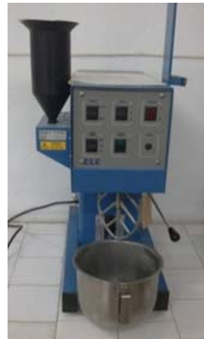
Fig. 1. Mortar mixer with manual/automatic functions according to SREN 196-1 produced by ELE company
