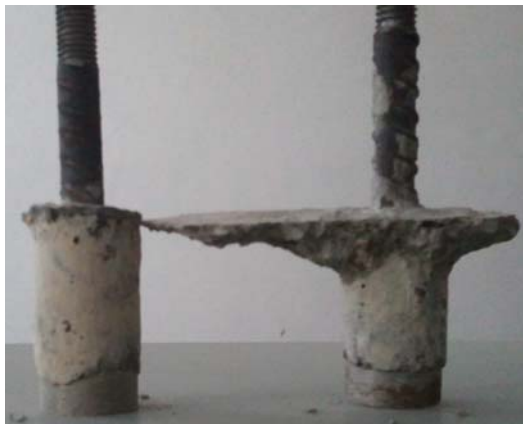
Fig.6. The pull-out connectors with (left) and no (right) steel plate confinement.
