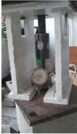
Fig.4. Developed tension test rig for confined tests
