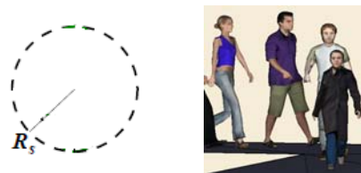
Fig. 7. The human body shape (left) and the visual representation (right) for agents used by Pathfinder
