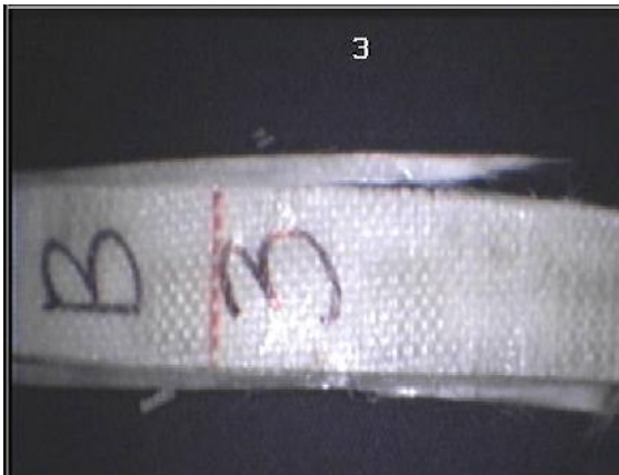
Figure 5 Specimen 3b Roving on weft magnified 5 times by video camera
