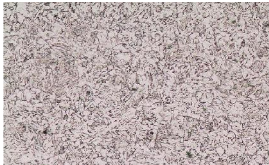
Figure 2. Microstructure of pipeline steel API 5L X65 (x100, nital etching).
