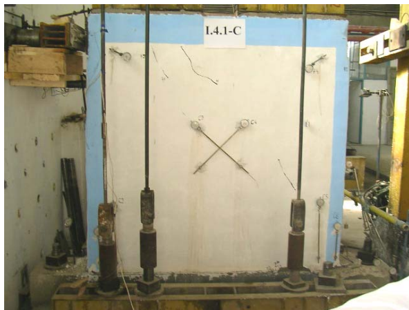
Fig. 4 Equipping of the trial stall for the consolidated masonry element
