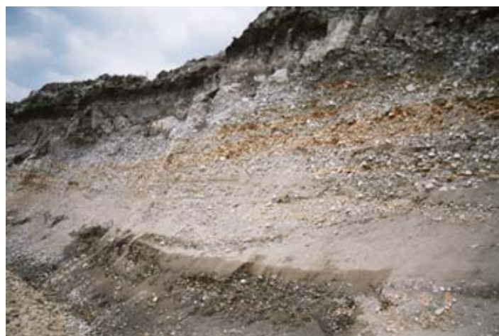
Fig. 3 Infiltrations in the sandy clay stratum
