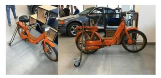
The second solution was with a support with 4 wheels under the moped and this was a good solution for our necessities
