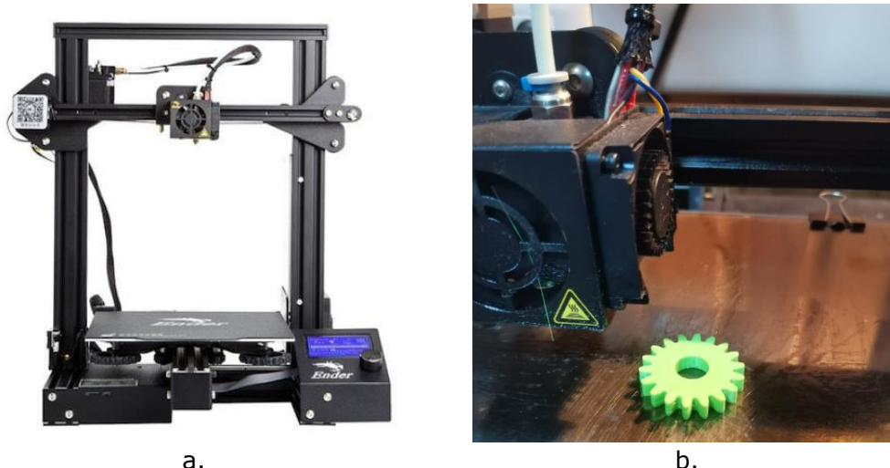
Figure 2: 3D printer (a. general view; b. image during the manufacturing process)
