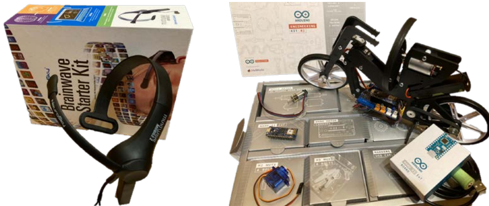
Figure no.1. The NeuroSkyMidwave Mobile headset (left) and the Arduino Motorcycle (right)
