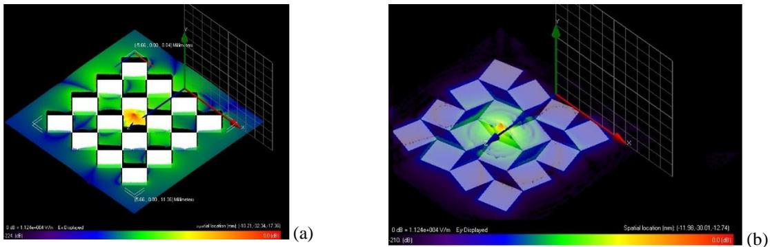
**Figure 2:** FDTD simulations results: (a) multiple periodic UCs and (b) RSD
