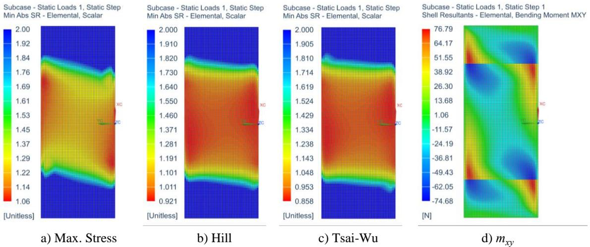
**Figure 6:** Minimum absolute values for SR (cross-ply laminate  $[45_3/-45_3]_S$ ), relative to the fringe plot of internal twisting shell moment ( $m_{xy}$ ) - FEA-based
