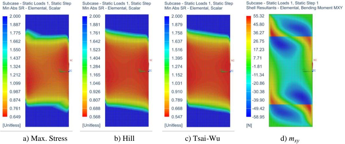
**Figure 5:** Minimum absolute values for SR (unidirectional off-axis  $[45_{12}]_T$ ), relative to the fringe plot of internal twisting shell moment ( $m_{xy}$ ) - FEA-based
