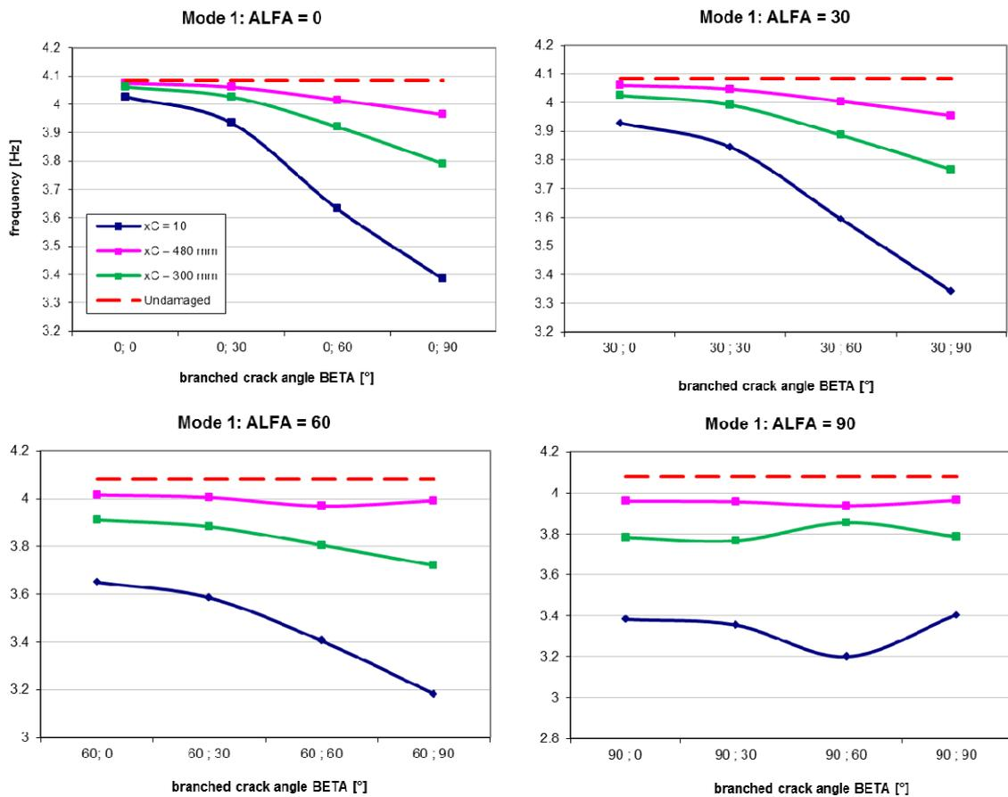
**Figure 4:** Plotted frequency shift curves for the first mode of vibration for the three damage positions
