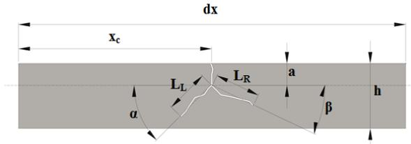
**Figure 1:** The geometry of the Y-shaped crack
