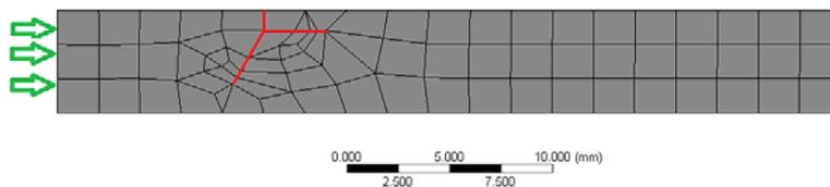
**Figure 2:** Zoom on the left fixed beam end highlighting the created damaged
