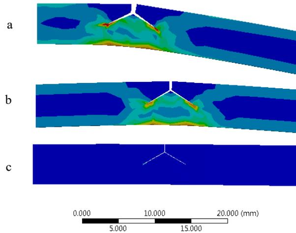
**Figure 3:** Zoom on the three characteristic locations: (a) maximum curvature at  $x_c = 10$  mm; (b) local maximum of the curvature  $x_c = 300$  mm; (c) curvature's inflection point  $x_c = 480$  mm
