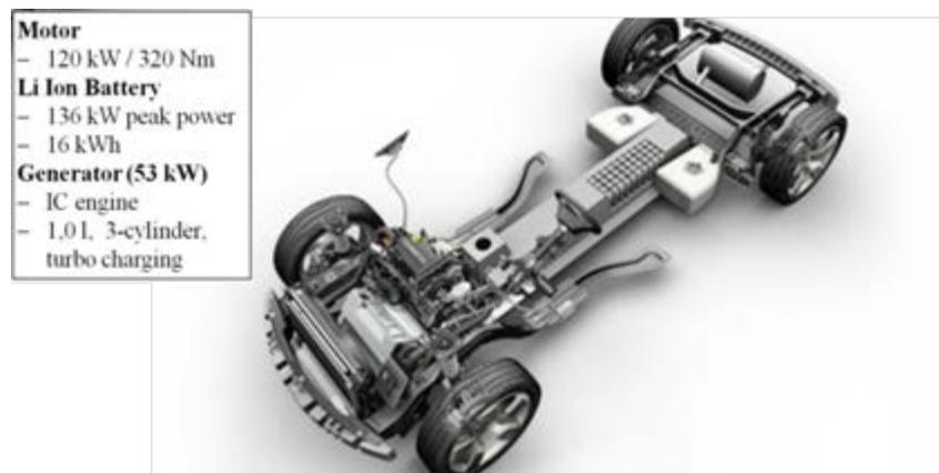
Fig. 2 – Four-stroke spark ignition engine as current generator for motor propulsion: Chevrolet E Flex Volt prototype (source: General Motors).
