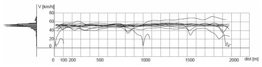
Fig. 8 – Speed versus distance diagram for multiple passes on the road segment A.
