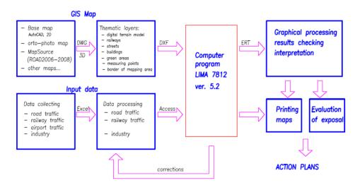
Fig. 1 – General diagram of noise mapping.
