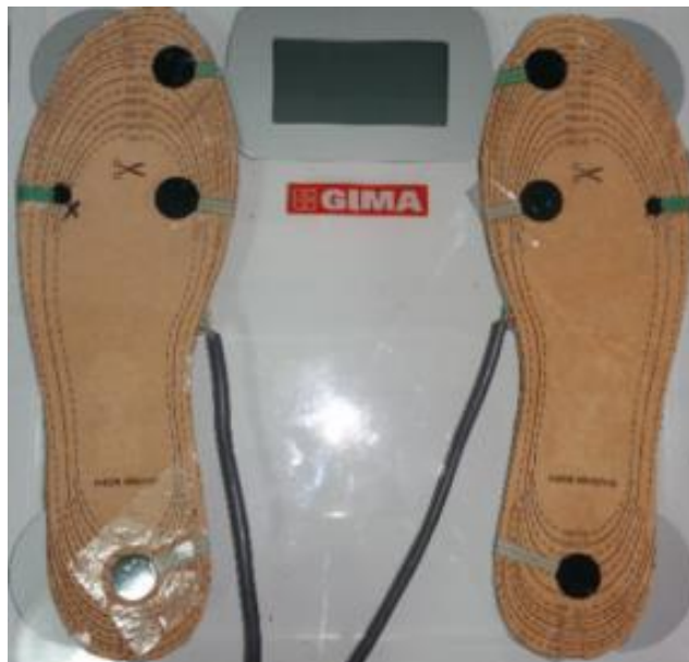
Figure 4: Soles with the corresponding sensors on the scale.
