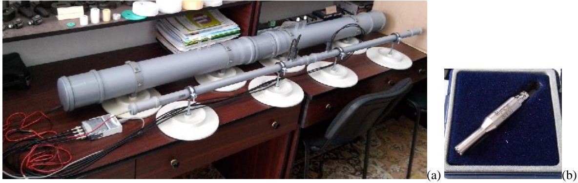
Figure 2: Experimental setup for sound transmission loss measurements: the large/small tubes (a) and the acoustic transducer – microphone (b)
