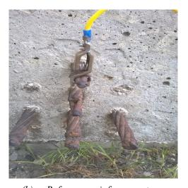
(b) Reference reinforcementFig. 2 (a, b). Using a Half-cell potentiometer
