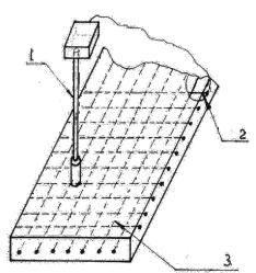
1. Half -cell potentiometer; 2. Reference re-bar; 3. Tested element Fig. 1. *Half -cell potential circuit*
