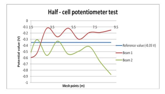
Fig. 4. Beams corrosion results
