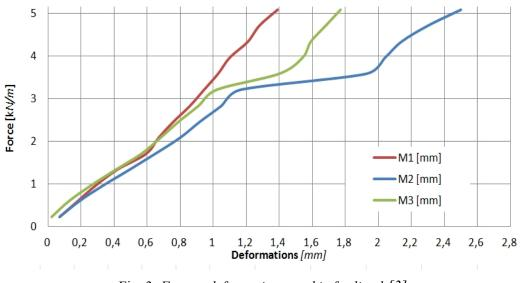
Fig. 3. Force - deformation graphic for lintel [3]
