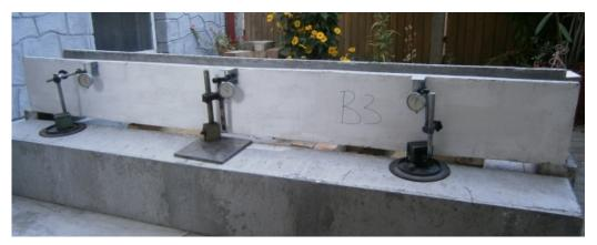
Fig. 1. Lintel ready for testing
