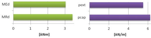
Fig. 5. Comparison between theoretical and actual capacity of the lintel
