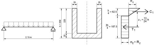
Fig. 4. Lintel calculation scheme
