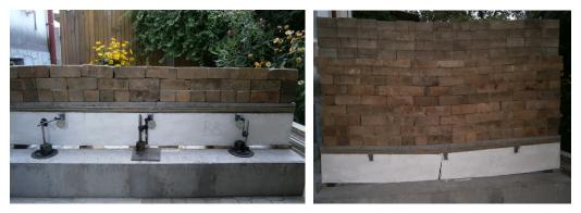
Fig. 2. Lintel during test and failure moment
