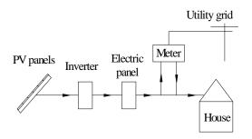
Fig. 1. Schematic diagram of the system
