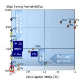
Fig. 1. Ozone Depletion Potential and Global Warming Potential [12]
