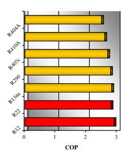
Fig. 3. COP values for different refrigerants for an air-water heat pump (A2/W35)
