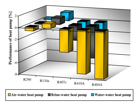
Fig. 6. The performance of different heat pumps as compared with those using R-22
