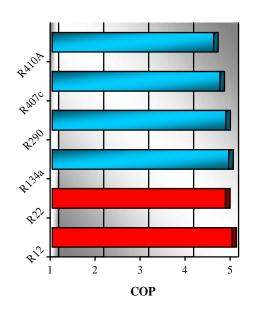
Fig. 4. COP values for different refrigerants for a water-water heat pump (W10/W35)
