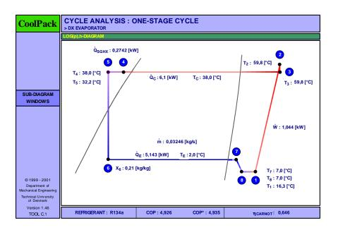
Fig. 2. Detail of the cycle analysis for a water-water heat pump (W10/W35) with R134a [6]
