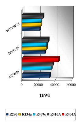
Fig. 7. The values of index TEWI for various refrigerants and different types of heat pumps
