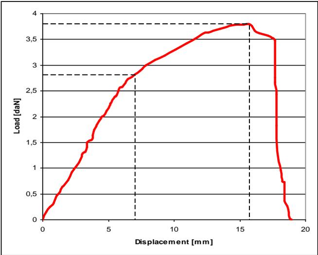
**Figure 7:** The Force-sag diagram to the specimen no. 1
