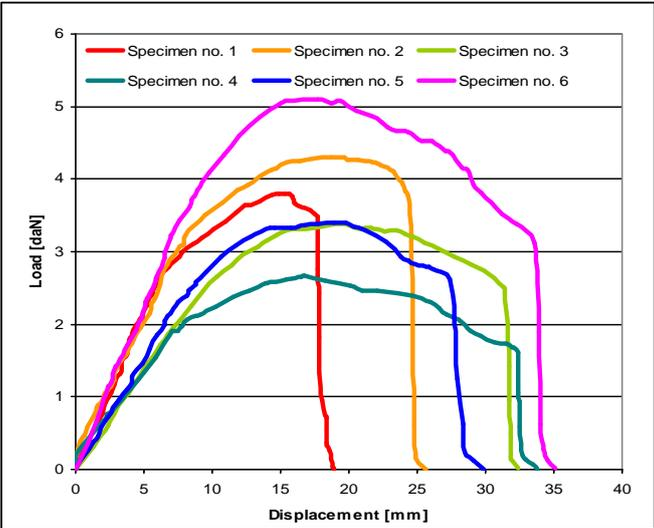
**Figure 8:** The Force-sag diagram to the specimens no. 1-6
