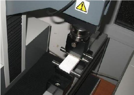
**Figure 5:** Settlement of the specimen
