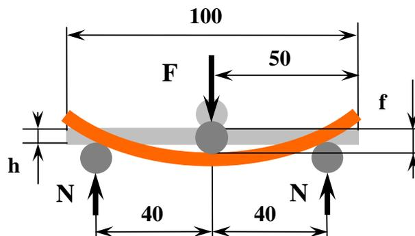
**Figure 1:** The scheme of the bending test of specimen
