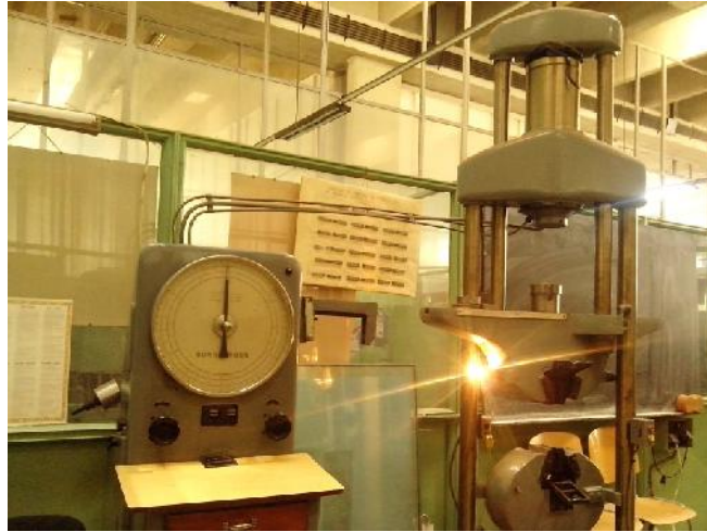
Figure 3: Bending test of experimental samples composite experimental NdFeB magnet sample using a hydraulic universal material testing machine model WE60.
