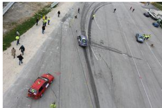
Fig. 1. End position of the cars after impact.
