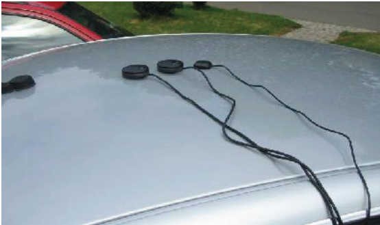
Fig. 12. The three GPS antennas on the vehicle roof
