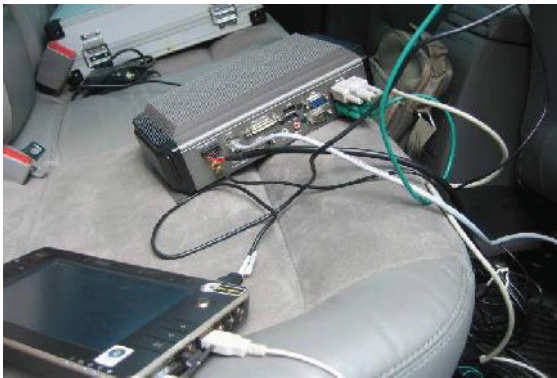
Fig. 13. The logging system (Trek-550 back panel with multiple RS-232 ports, assisted by a tablet-pc as smart display)
