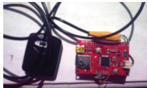
Fig. 6. Mod-GPS connected to Logomatic v2
