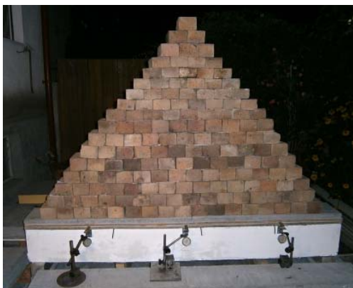
Fig. 4. The final load with the 17th row of bricks
