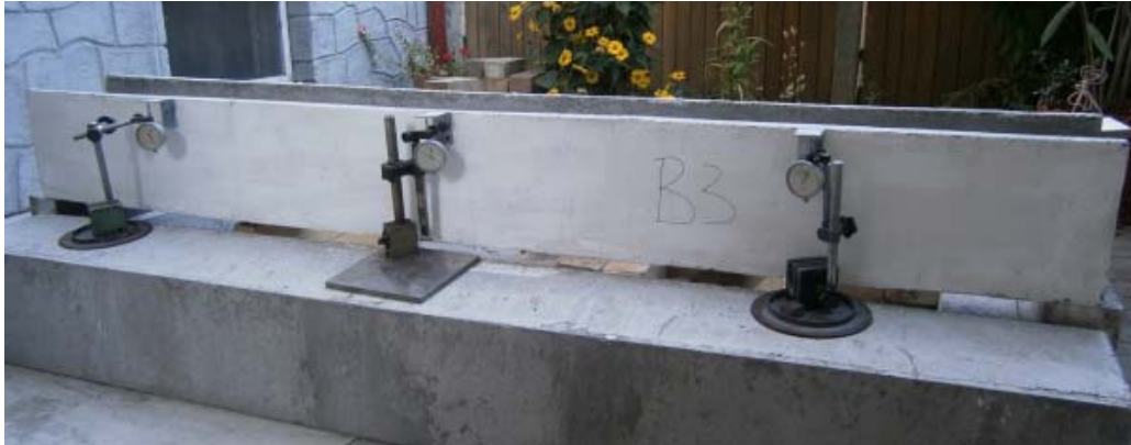
Fig.5. B3 lintel ready for testing
