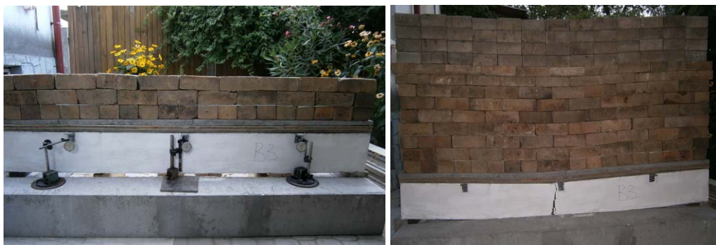
Fig.6. B3 lintel during test and failure moment
