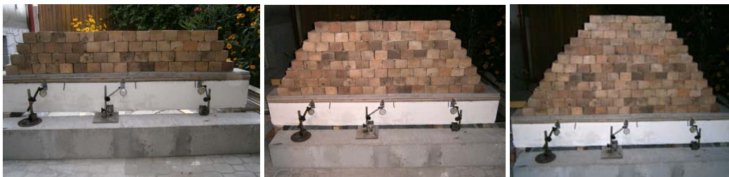
Fig.3. Increasing load with 4, 8, 12 rows of bricks
