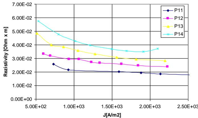
**Fig. 4** Electrical resistivity variation with the current density (J) for a representative samples for each class of particle reinforced composites developed and tested
