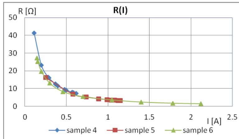
**Fig. 2**  $R(I)$  dependence for conductive composite samples having different volume fraction of carbon and iron particles
