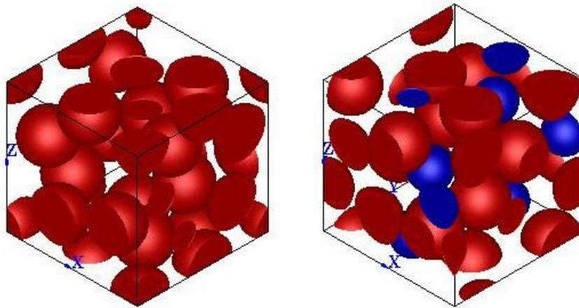
**Fig. 3** Representative volume elements for random particle reinforced polymeric composite (left) and multiphase particle-particle reinforced polymeric composites (right)
