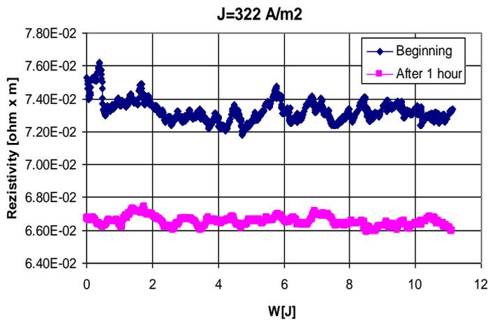
**Fig. 5** Resistivity variation with the energy applied in case of the 65% Fe, 15% C and 20% polymer composite – to time instants (1 hour shift)
