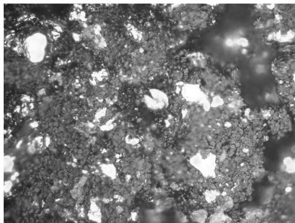
**Fig. 1** Optical microscopic view (x500) for a 70% Fe, 10% C and 20% polyvinyl acetate polymeric composite material
