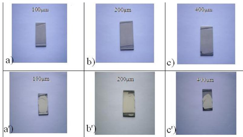
**Figure 2:** Samples with the coating thickness of 100 μm, 200 μm and 400 μm before and after the thermal shock test at 1200 °C: a;b;c- before thermal shock test; a';b';c'- after thermal shock test at 1200°C
