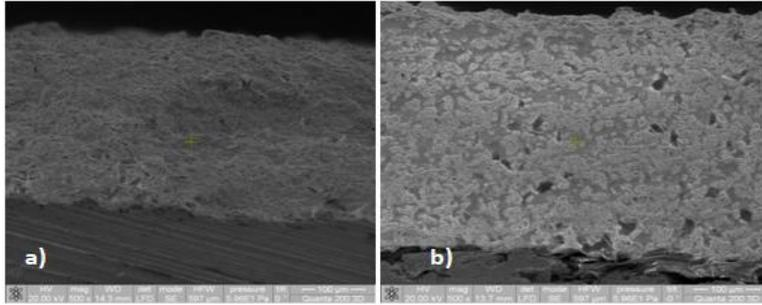
**Figure 8:** SEM images in cross-section of the YSZ coating: a) before the thermal shock test; b) after the thermal shock test.
