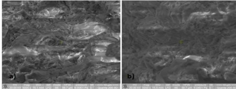
**Figure 9:** SEM images in cross-section of the YSZ coating: a) before the thermal shock test; b) after the thermal shock test.
