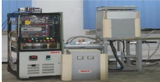
**Figure 1:** QTS2-Installation for material testing in extreme thermal conditions
