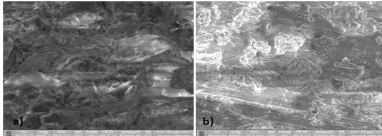
**Figure 13:** A SEM cross-sectional image which shows the microstructures of the YSZ surface layer: a) before the heat shock test, b) after the heat shock test.
