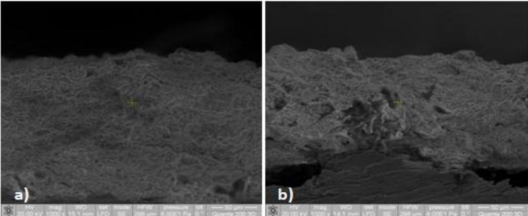
Figure 5: SEM images in cross-section of the YSZ coating: a) before the thermal shock test; b) after the thermal shock test
