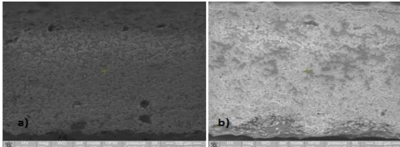
**Figure 12:** A SEM cross-sectional image which shows the microstructures of the YSZ surface layer: a) before the heat shock test, b) after the heat shock test at a temperature of 1200  $^{\circ}\text{C}$ .
