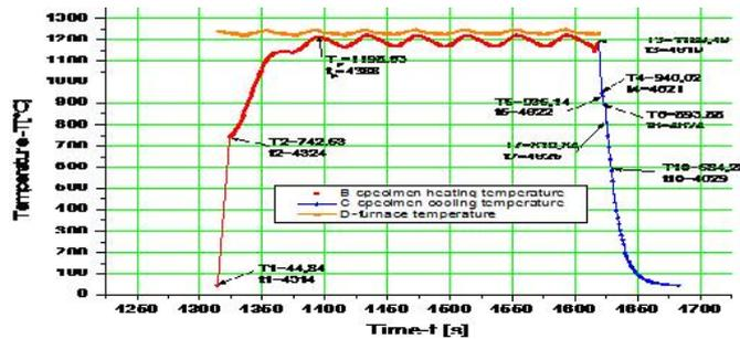
**Figure 10:** The graph resulted from the heat shock test conducted at a temperature of 1200 ° C for the sample with the coating thickness of 400 µm
