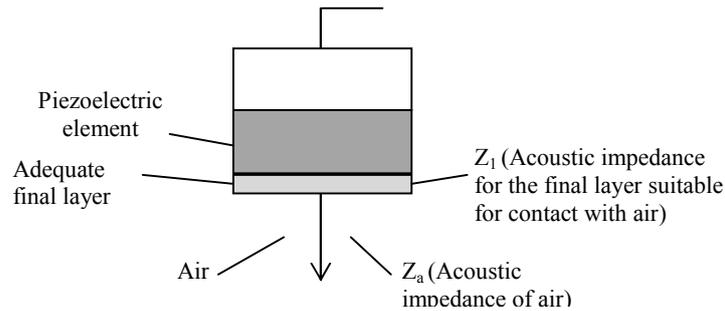
**Figure 2.** An ultrasonic transducer diagram indicating adequate final layer of acoustic impedance relative to critical and piezoelectric coupling medium, air.
