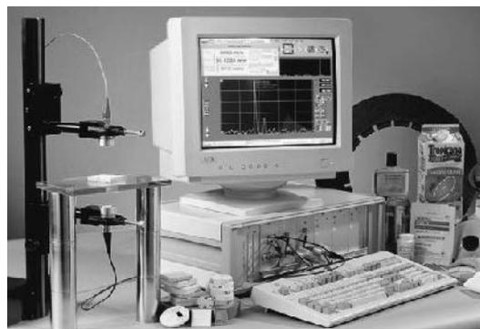
**Figure 3:** Stand SECU 01-FC experimental model of non-contact ultrasonic testing, which uses contactless sensors and a screen that displays the material thickness and speed testing
