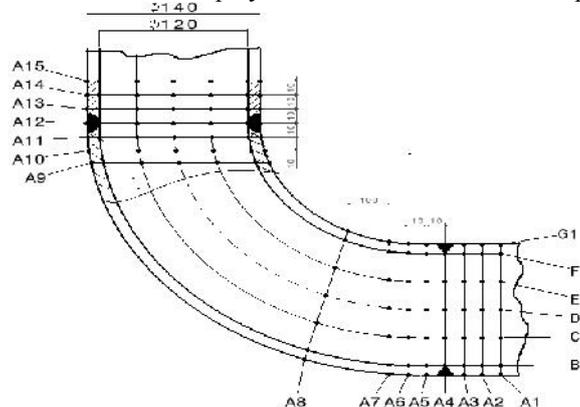
**Figure 4:** Ultrasonic control scheme of an elbow 90°:
