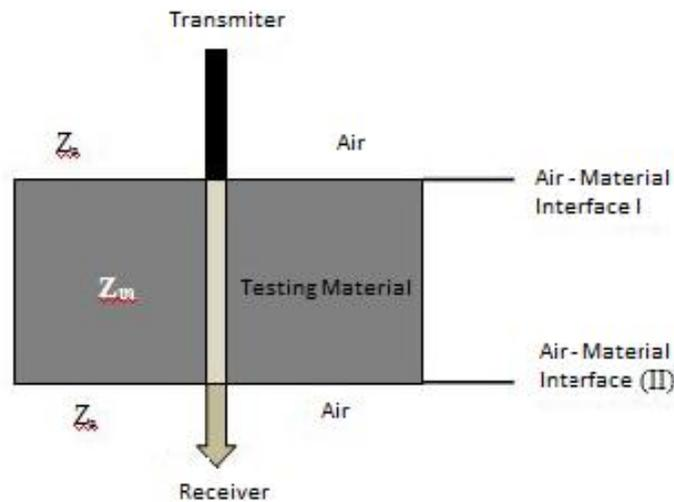
**Figure 1:** Areas to be traversed by ultrasound (shown by arrow) in non-contact mode of transmission ultrasound to propagate through a material testing.
