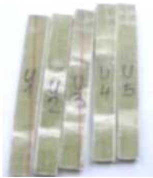
Figure 2 Specimens Roving 4 layers on warp
