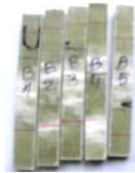
Figure 3 Specimens Roving 4 layers on weft
