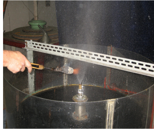
Fig. 9. Flame behaviour in the contact with the two-phase jet
