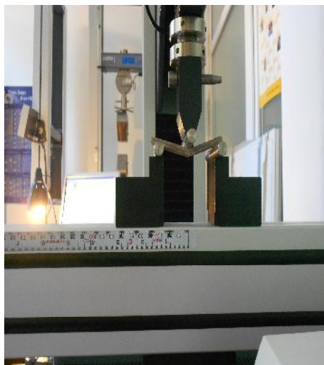
Figure 2. TA Plus materials testing machine in a three-point bend test
