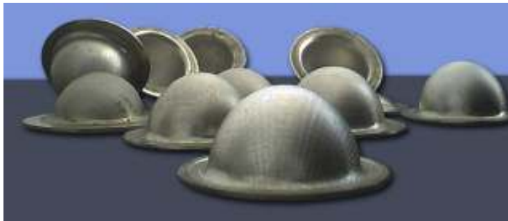
Figure 1 – Gasostatic deep drawing samples
