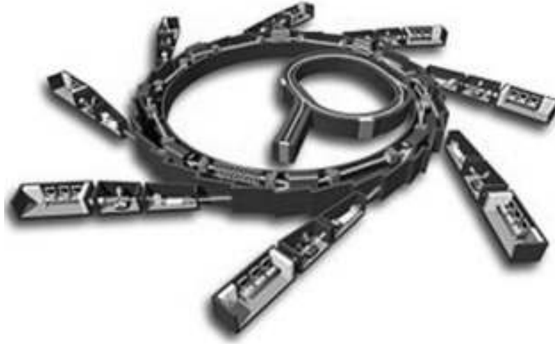
Fig. 2: A high energy synchrotron schema
