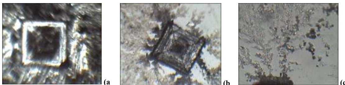
Fig. 5: The salt crystals structured in static magnetic field ( b and c ) have similar shapes with the ones structured in neuter environment ( a ). There is still a significant difference observable for not crystallized remains
