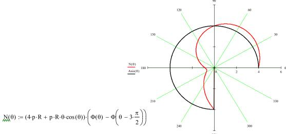
Fig. 7. Axial force diagram in polar coordinates
