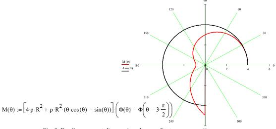
Fig. 8. Bending moment diagram in polar coordinates
