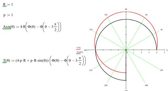
Fig. 2. Shear force diagram in polar coordinates
