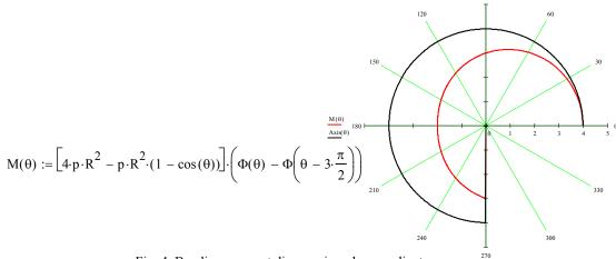
Fig. 4. Bending moment diagram in polar coordinates
