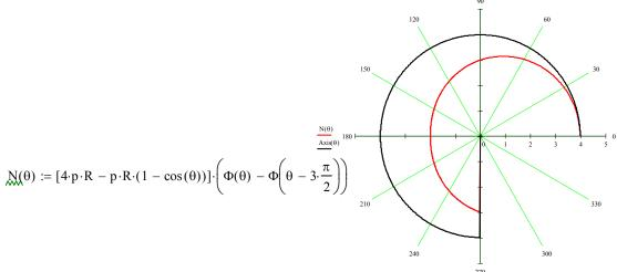
Fig. 3. Axial force diagram in polar coordinates
