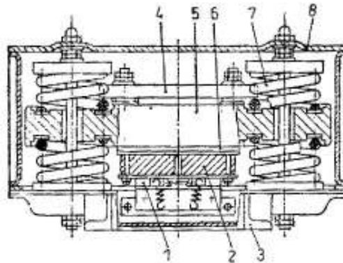
Figure 3. Construction of electromagnetic vibrator
