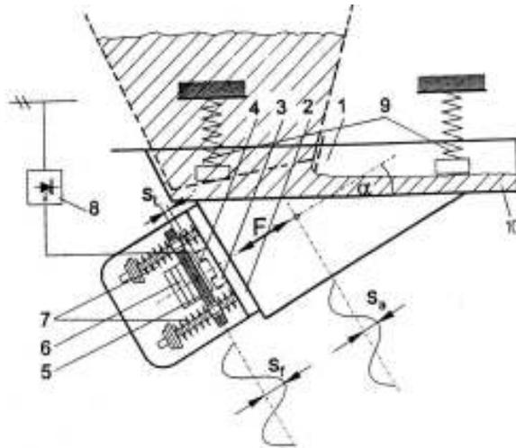
**Figure 5.** Magnetic vibration feeder: 1-vibration flute; 2 - vibrator housing and other components; 3-electromagnet; 4- mobile magnetic coreplate; 5, 6- additional masses; 7 - spring;8 - control device; 9- suspension springs;10- transported material.  $S_f$  - vibration amplitude (free side);  $S_a$  -vibration amplitude (working side).
