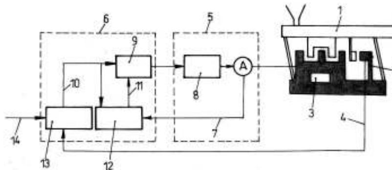
**Figure 7.** Combined control of vibration amplitude and resonance frequency: 1 - vibration feeder; 2 - vibration transducer; 3 - magnetic drive; 4 - feedback signal; 5 - power unit; 6 - control system; 7 - current signal; 8 - amplifier; 9 - AD converter; 10 - set-point amplitude; 11 - set-point frequency; 12 - frequency control (slow); 13 - amplitude control (fast); 14 - input signal
