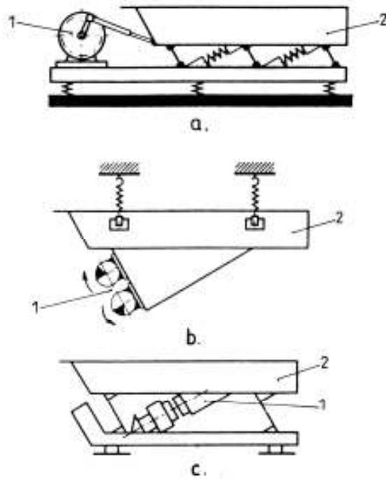
**Figure 1.** Basic types of vibrating feeders: a-with rod-cran mechanism; b-with eccentric mass; c- with electromagnetic vibrator: 1-vibration generating mechanism; 2- vibrating mass with transporting chute.
